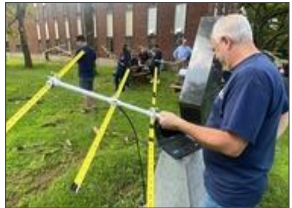
The teachers made tape measure Yagi antennas for the experiment. [Sierra Harrop, W5DX, photo]
