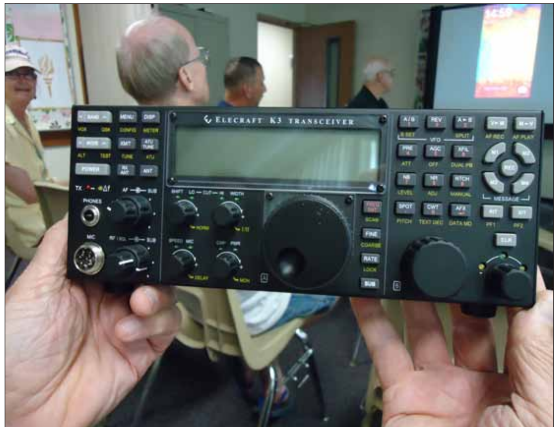
Joe passed around the analog portion of an Elecraft K3 to show how a laptop/usb cable/analog K3 combo will let an operator get connected without a modem. Using a smart phone, Joe demonstrated how he can connect with the Web DX KH6 station on Oahu. He wasn't able to connect at that time, but says he has worked it successfully, even "while taking a bath." He also demonstrated the CW link. For more details, visit http://www.remotehamradio.com .
