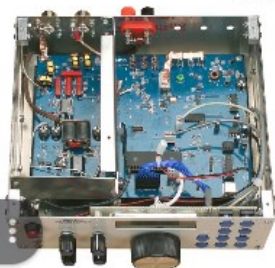
A compact competent transceiver covering 12, 10 and 6 meters, designed and built by Jim Veatch, WA2EJ
